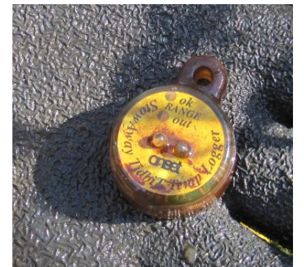
This thermograph was recently removed from Bee Creek in Minnesota, one of five sites in the watershed where the devices were installed this year. The thermographs were attached to heavy stakes, which were pounded into the streambed.
